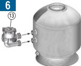
Mount the multiport valve. Position the bottom throughwall flange first, then the upper one. Tighten the nuts moderately.
