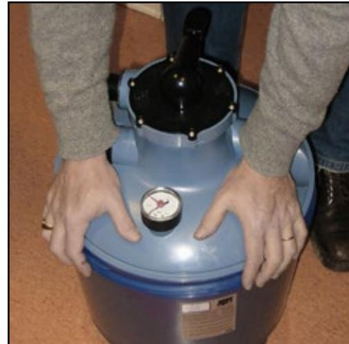
Bear down simultaneously with both hands to push the lid completely into the filter tank. Maintain pressure on the lid until the ring is screwed into position.
