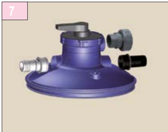
Gluing the unions onto the lid: The transparent union is joined to the waste outlet, the black union to the inlet and the 3 piece union to the outlet on the 'pump' side.
