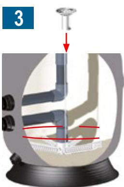
Pour the sand (granulometry 0.6/1.25) in carefully to avoid damaging the laterals. Remove the tape and put the diffuser back in position.
