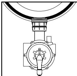
**FILTRATION** : The usual valve position. Water from the pump crosses the filter from top to bottom and returns to the pool.
