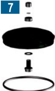
Assemble the air bleed valve on the lid.
