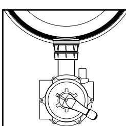
**RINSE** : Water from the pump passes through the filter from top to bottom and is then routed to waste.
