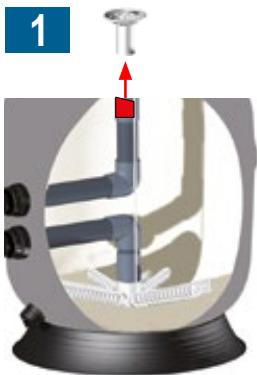
Remove the diffuser and cover the opening of the tube with adhesive tape.
