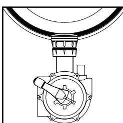
**CLOSED** : No circulation is possible. Never run the pump while the valve is in this position.
