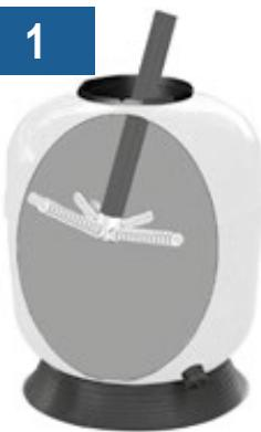
Pass the collector pipe into the filter and screw on the laterals, be careful not to over tighten.
