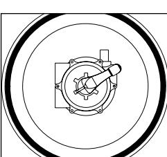
**CIRCULATION :** Water from the pump returns directly to the pool without passing through the filter.
