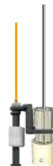
Step 20 (option) Mount the level sensor and its ballast and adjust it.
