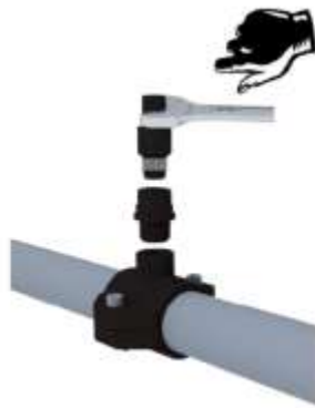
Screw the union onto the saddle clamp
