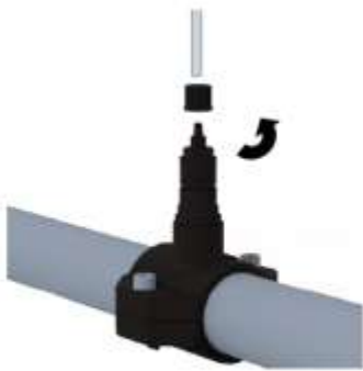
Loosen the injection valve nut.
