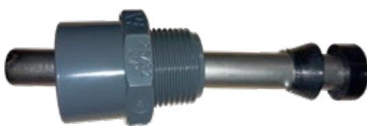
Remove the straight part of the seal from the thermowell before fitting it into the threaded port. Only retain the conical section of the seal.
