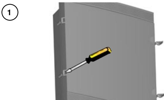
Remove the hinges and the locking plates
