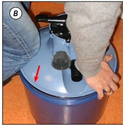
Press the lid into the filter tank at one point. Using your knee, maintain pressure on this point
