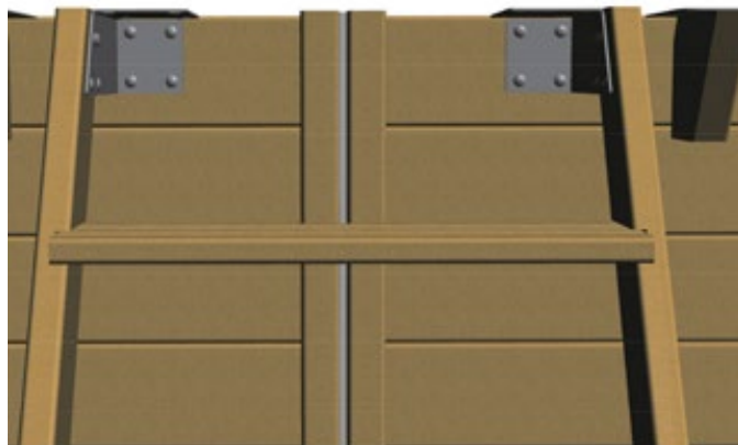
Figure 18 – Fastening the access ladder to the pool wall
