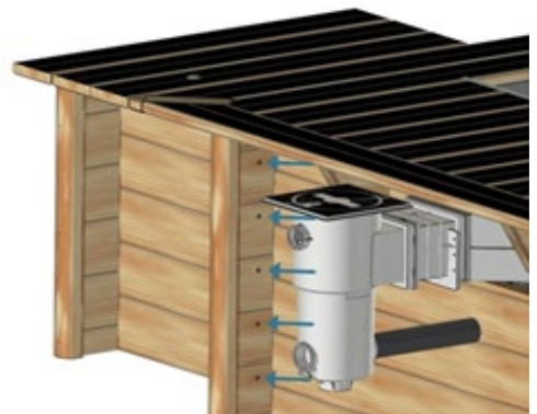
Figure 64 – Fastening the cover pit to the pool
