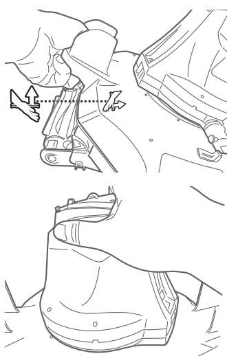
**CLEANER RETRIEVAL NOTE:** For roller version, retrieve the robot from the pool surface by grabbing onto the fin and swivel head. Be sure to always grab the fin on the side with the hand symbol (see image) to prevent debris from falling into the pool during retrieval.
