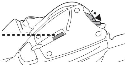
3. Slide the power switch to “ON” ( while the robot is still submerged ) – the indicator light will turn on and activate the motor automatically ( water level covering the sensors at the top of the swivel head ). Let the robot sink to the pool floor and observe its first forward and reversed movements across the pool bottom. If it runs along the pool wall instead of perpendicularly, retrieve it and redeploy it while making sure its front/back is facing the pool wall.
