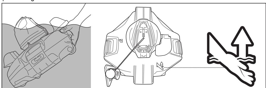
5. Slide the power switch OFF. Rinse the robot with fresh water after every use. DO NOT use any detergent.
