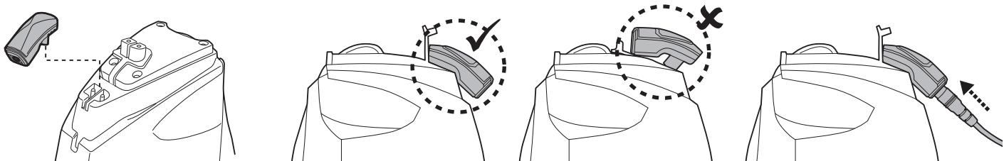
3. Connect the external adaptor to the power source. The indicator light on the external adaptor turns red once the charging begins. The indicator light on the external adaptor will turn green when the robot is charged.
