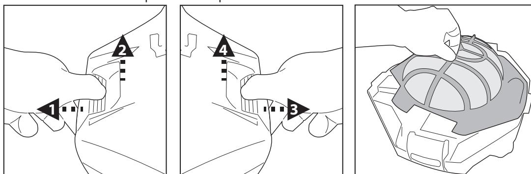
2. Detach the filter cover and remove the debris from the compartment. It is recommended to clean the filter cover net with splashing water. If brushing is deemed necessary, use only a soft brush to clean it carefully and gently to avoid damages.
