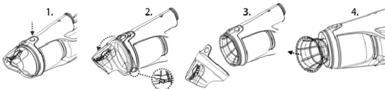
**CAUTION!** Replace the damaged filter cage immediately before the next operation.
