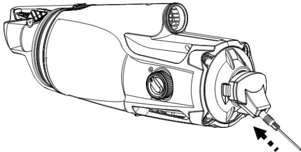
4. Connect the external adaptor to the power source. Once the pool vacuum begins charging, the indicator light on the external adaptor will turn red. Normally, it takes about 4-6 hours to reach a full charge. The indicator light will turn green when the pool vacuum is almost fully charged.
