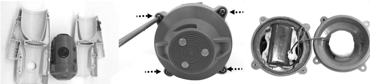
4. Use Philips screwdriver to unscrew screw on the corner of the supporting plate as pointed at. Use clamp to catch the plate and pull it out to expose the wire connectors on the PCB.
