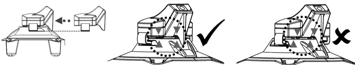
3. Plug the jack of the external adaptor into the charging port at the end of the charging base.
