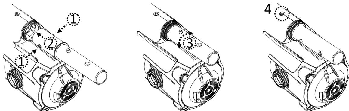
Slide the telescopic pole onto the pole connector. Press on the side pins of the connector and slide the telescopic pole further down until the pins of the connector are secured inside the holes of the pole.
