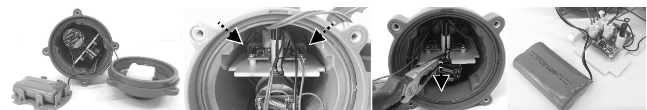
5. Locate the middle connector as indicated, press the clip on the connector and pull it out. NOTE: Wrap the connector immediately with insulating tape in order to avoid short circuit caused by the contact of both wire terminals.
