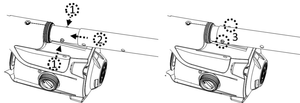
To release the telescopic pole, press down the side pins simultaneously and pull out the pole.
