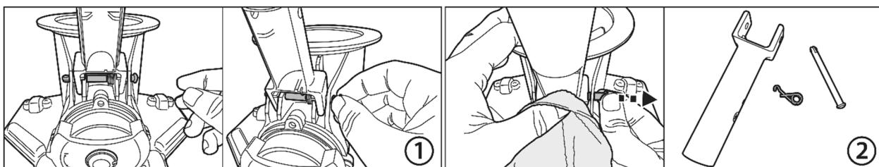
1. Grasp the top round end of the pin. Use a pair of pliers to help with removal if necessary.
