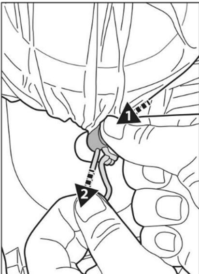
While holding the cord, press on the cord fastener and push it under the flange.
