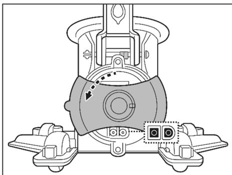
2. Align and attach the charging cable to the charging port. **WARNING!** Be sure not to invert the charging cable and ensure both the charging cable and charging port are clean and dry before charging them. TIPS: Use cotton bud to dry the charging port and pins. Connect the external adaptor's cable plug to the charging cable's port.
