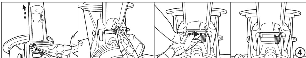
4. Use a pair of pliers to pull the hook from the bottom of the connector, then fix it onto the connector as shown. Move the entire spring to the right.
