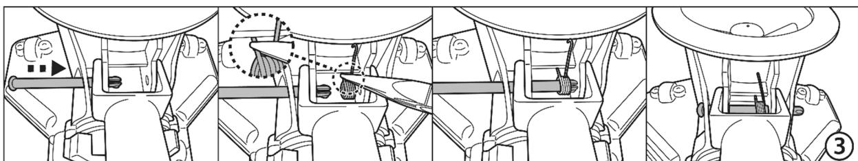
3. Insert the pin from one end and place the spring as shown with the help of a pair of pliers. Ensure the hook is on top and the other end is installed underneath the bench as shown. Align and insert the pin all the way through the spring hole and opposite hole.
