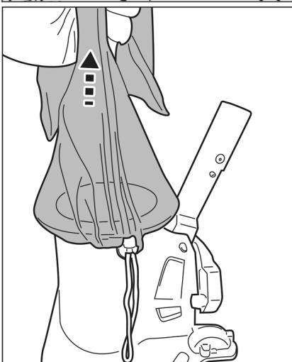
Lift up the bag to ensure it is totally secured before deploying the pool vacuum into water.
