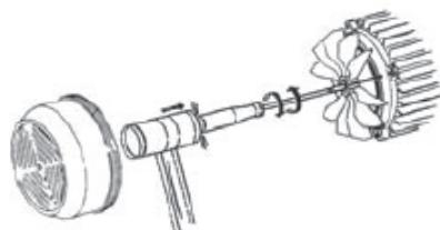
Check that the direction of motor rotation corresponds with that indicated on the specification plate (the fan should rotate in a COUNTERCLOCKWISE DIRECTION, when viewed from the rear of the motor. If the motor is three-phase and it is observed that it is rotating in the opposite direction, then two of the supply phases should be inverted at the protection panel.
