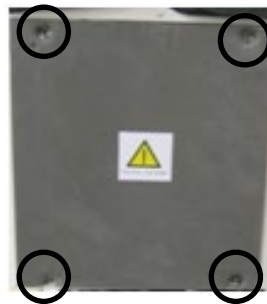
Extract the 4 screws from the lid of the box
