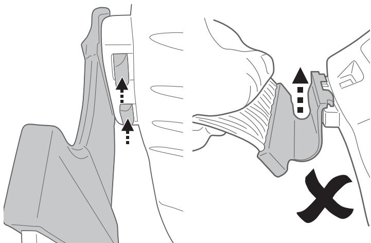
**TIPS:** Press on the two hook ends to remove the brush.
